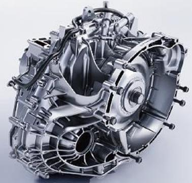
7-Speed Wet-Type Dual Clutch Transmission
